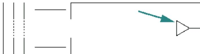
The detector which is usually a microchannel plate, must be operated below  $1 \times 10^{-5}$  torr. This usually determines the maximum allowable pressure in the flight tube.
