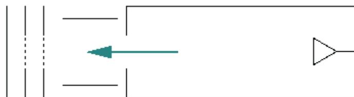
Often the source region is at a suitably low pressure. In this case the flight tube is pumped by the opening into the source region.
