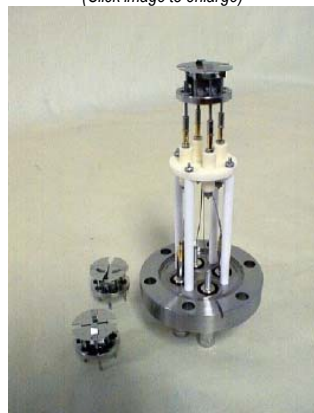
Egun Mounted on 2.75 Conflat Flange
