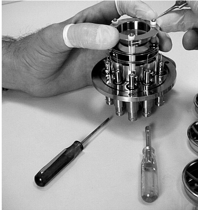
20. Place Input Grid over ceramic inserts and hold it down evenly with fingers while replacing washers and nuts. Alternately tighten nuts one turn at a time in a circular pattern until all are snug. Do not over tighten.
