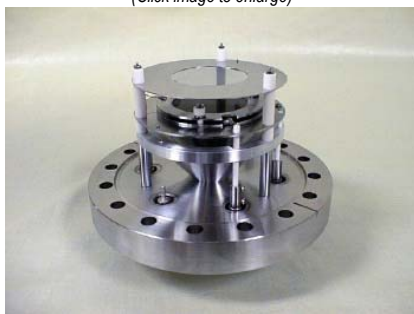
40mm MCP Dual Detector on 6 Inch Conflat Flange
