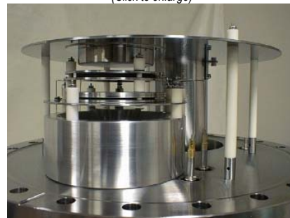
40mm Z-Gap MCP Detector Mounted on AREF (RETOF)
