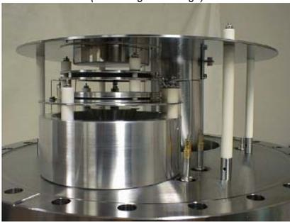
40mm Z-Gap MCP Detector Mounted on AREF (RETOF)
