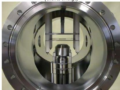
C-1551 Solid Sample Probe and Load Lock Assy
